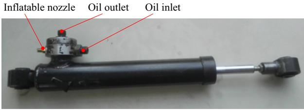
Fig. 8. Actuator prototype of the pumping regenerative damper.
